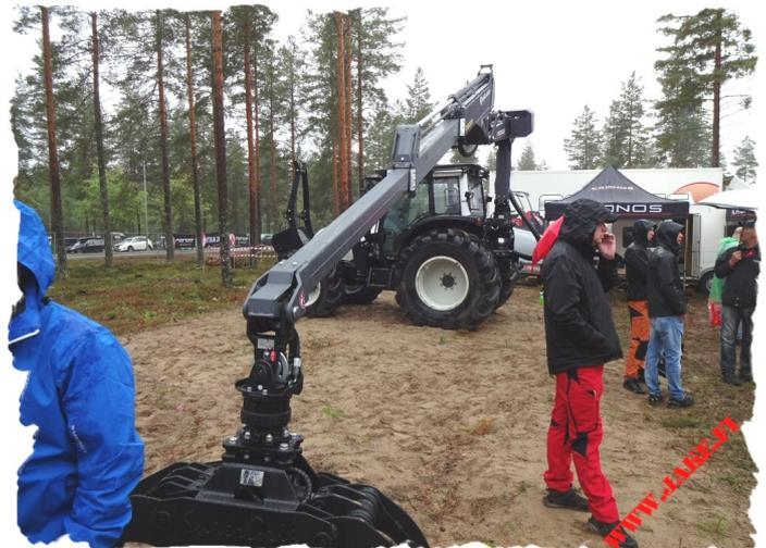
The **JAKE 900** makes using the crane versatile as the crane mounted on the tractor can be combined with other devices connected to a 3-point linkage and a trailer hitch usually with no limits (except for parallel cranes).
