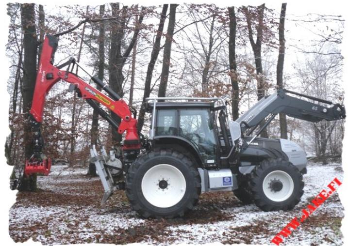
The **JAKE 800** makes using the crane versatile as the crane mounted on the tractor can be combined with other devices connected to a 3-point linkage and a trailer hitch usually with no limits (except for parallel cranes).
