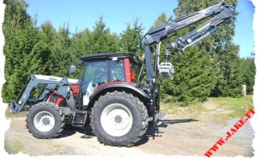
The JAKE 600 makes using the crane versatile as the crane mounted on the tractor can be combined with other devices and equipment connected to a 3-point linkage and a trailer hitch usually with no limits.
